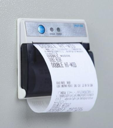
Maxim PNP-64 is loaded from the front and is well suited for manned applications where trained staff use a device or instrument. It is regularly used in building control panels, diagnostic equipment, medical devices, measuring instruments and much more. PNP-64 features a robust SST IC powering multiple baud rate and high input buffer. It also features an extremely rugged and high speed printer mechanism with a tough body.
